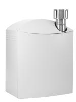
The Cloud Droplet Analyzer is a high-resolution optical aerosol spectrometer optimized for measuring size distribution and number concentration of cloud aerosols like droplets and ice crystals.
