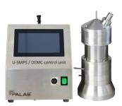
The DEMC size classifier (as defined in ISO 15900:2000) selects aerosol particles from an aerosol stream according to their electrical mobility. Different lengths of columns are available depending on the size range to be selected. Depending on the configuration of the control unit and column, the designation changes accordingly.
