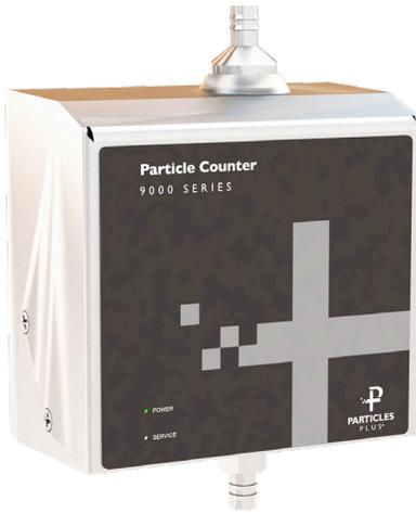
The 9510 particle counters provide a range of particle size measurement from 0.5 to 10.0  $\mu\text{m}$  at a flow rate of 1.0 CFM (28.3 LPM). These sensors allow for efficient particle counting with specifications that exceed the ISO 21501-4 and JIS B9921 calibration standards.
