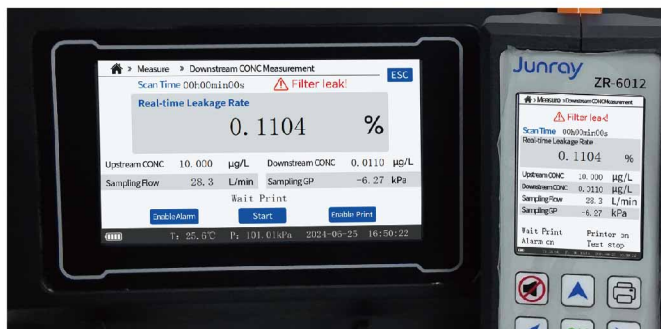
The synchronized photometer and filter scanning probe ensures easy control when scanning filters with all the information at your fingertips.
