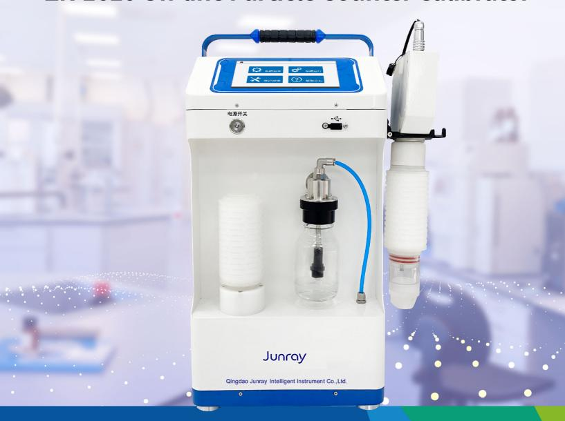
ZR-1610 On-line Particle Counter Calibrator is used for detecting and calibrating the on-site online airborne particle counter.
