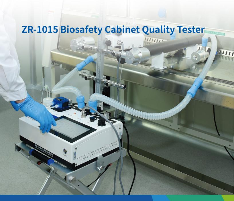
ZR-1015 Biosafety Cabinet Quality Tester is used to test the protection performance of class II biosafety cabinet by potassium iodide method. Different from the usual microbiological methods, potassium iodide test method can be counted on site to verify the protective performance of the biosafety cabinet: The usual microbiological method takes 48 hours; and potassium iodide test method takes only 30 minutes, which will not pollute the laboratory environment.
