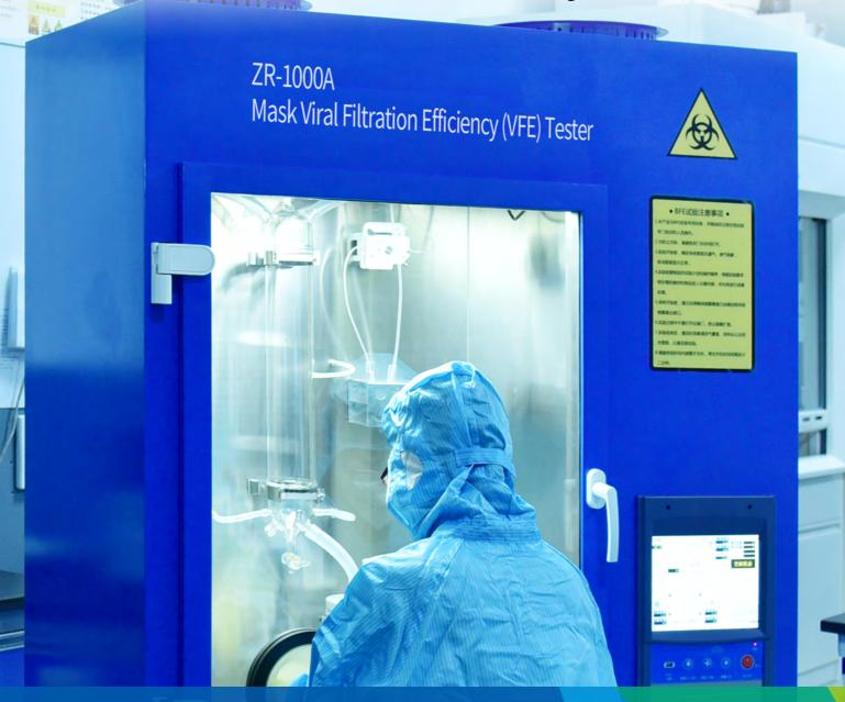
The Viral Filtration Efficiency (VFE) test determines how well a mask filters virus-containing droplets about 3 microns in size. It is similar to BFE in that it uses droplets of similar size, but uses a different challenge organism (bacteriophage instead of bacteria).
