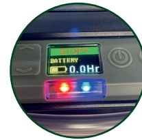
OLED full colour display with Red/ Blue LED's to indicate pump status, visible from a distance
